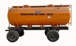
The oil tank is horizontally mounted on wheels equipped with inspection manholes & gauge glasses. The tank can also be provided with suitable saddles so that it can be rested on ground after removing from the trolley. All tank vents are fitted with dehydrators to prevent the entry of moisture into the tanks. The oil tanks shall be vacuum tested and for leakage as well.
