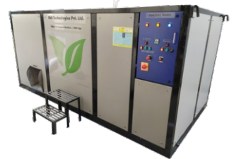
Shredder + Electrical Dehydration
